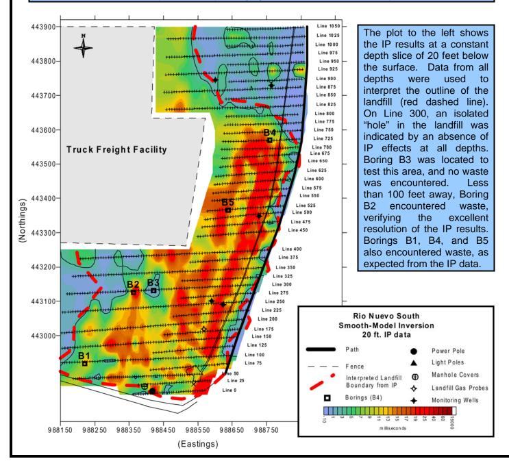
Depth of soil cover and depth of waste material can both be determined using the IP method. The figures below display the trenching results in plan view and in cross section from a buried landfill in Tucson, Arizona. Shallow trenching on the western portion of the area did not encounter any buried waste material, whereas trenching on the eastern half showed waste from a few inches to several feet below the surface.
