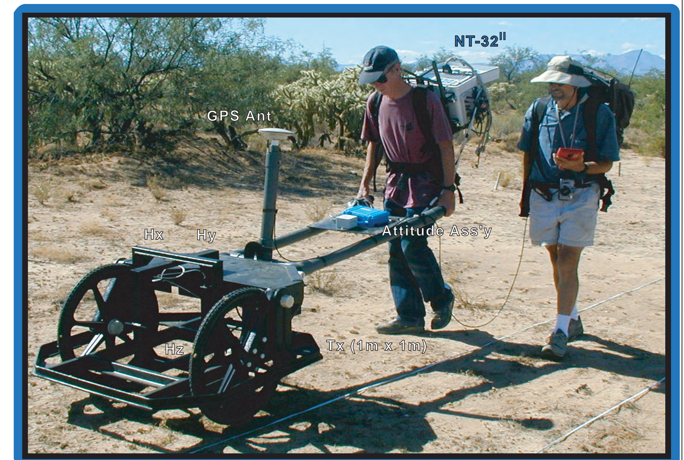
DNT System at Zonge / University of Arizona UXO Test Site
