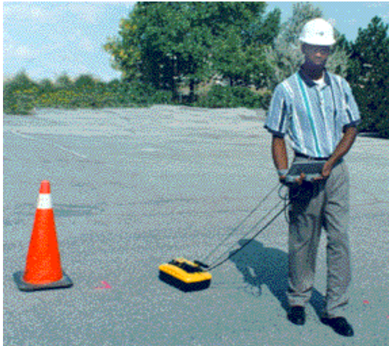
Figure 7-22. A GPR system in use. The system shown here is the Noggin 500 system, which operates in the 250 – 750 MHz range, and is designed for high-resolution imaging of the shallow subsurface (up to 8 meters depth, depending on materials). The system is manufactured by Sensors & Software, Inc. of Mississauga, Canada. (Figure courtesy of Sensors & Software, Inc.)
