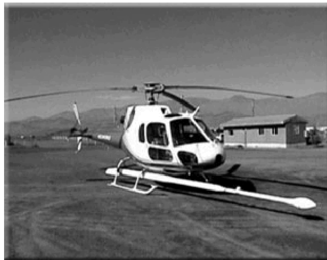
Figure 7-4. Fugro Airborne Survey's helicopter-borne stinger mounted magnetic sensor system (courtesy of Fugro Airborne Surveys).
