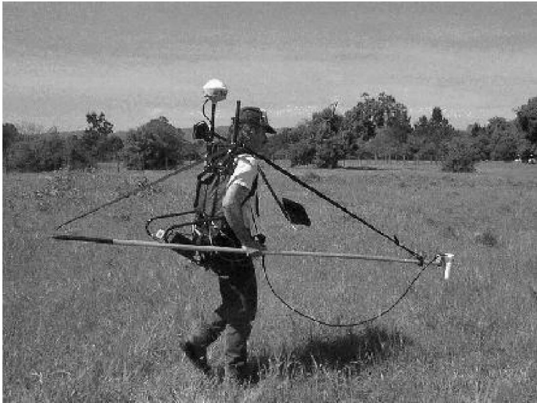
Figure 7-3. A Geometrics 858 Mag Mapper portable ground magnetometer with integrated Trimble GPS positioning system (courtesy of Geometrics).
