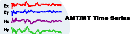
NSAMT measures changes in the electric and magnetic fields with time.
