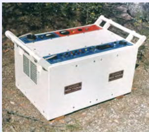
Transmitter used in IP surveys.
