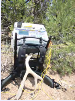
GDP32– multichannel receiver manufactured by Zonge
