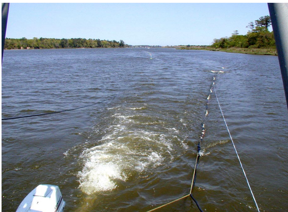
Figure 4. Resistivity streaming in Indian River Bay. Resistivity streamer with floats distant left. Seismic streamer (short) on right. The powerboat (USGS Storrs) and a University of Delaware (Newark) pontoon boat supporting the seismic gear are temporarily lashed together to steam in tandem
