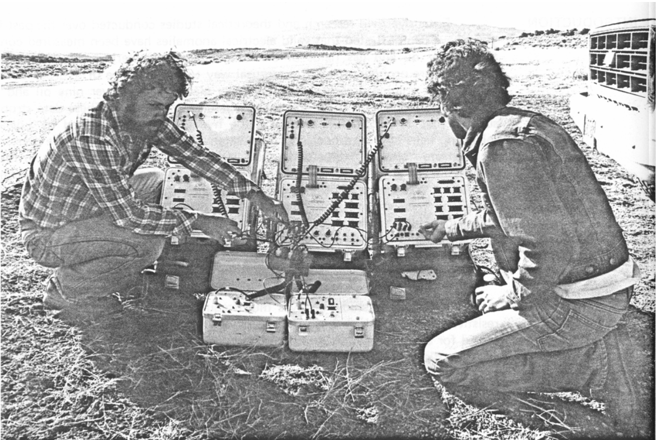
Figure 1. Equipment calibration and check prior to data acquisition at Lisbon Field. The field work involved a crew of eight, operating three backpack-mounted receivers simultaneously. Present-day surveys require smaller crews.
