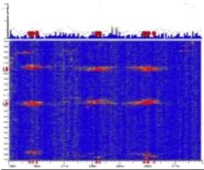
A screen shot of the Helios system output captured while two horses ran across the buried fiber-optic cables. The red traces are clearly visible, unlike those made by a small dog, and also quite distinct from the traces created by humans, cattle or trucks.
