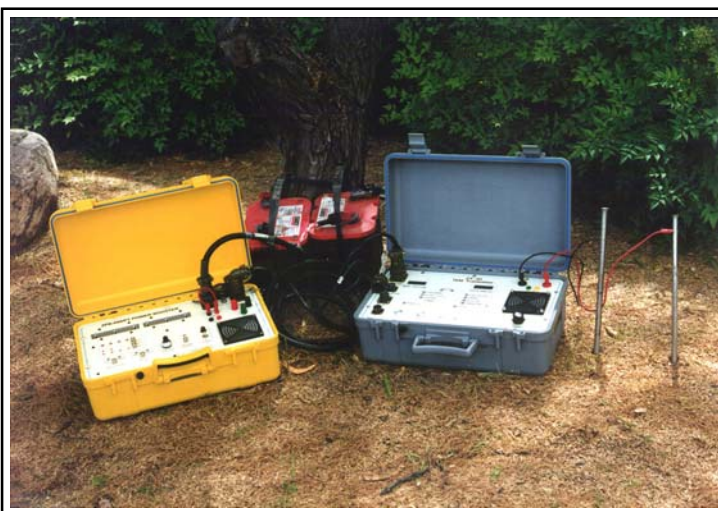
Figure 1: Functional block diagram showing a battery-powered Resistivity/IP system consisting of a ZPB-600 / ZT-30 Transmitter together with a Zonge GDP-32 Receiver.
