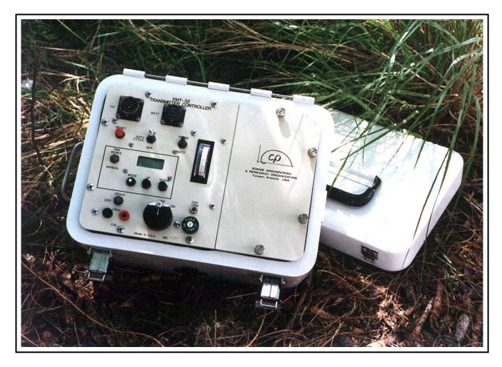
The XMT-32S Transmitter Controller produces timing signals for controlling all of the Zonge Engineering GGT, ZT and NT transmitters. Provision is made for synchronizing multiple controllers and GDP receivers. Frequency control can be accomplished either manually or by a time sequence program which is loaded through the RS-232c port. Time sequence status and frequency are displayed on an LCD on the front panel.
