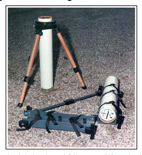
The TEM/3 antenna is a single channel magnetic field antenna useful for transient electromagnetic (TEM), controlled source audio-frequency magnetotelluric (CSAMT), and other types of EM geophysical surveys measuring vertical or horizontal fields. Multiple units may be used simultaneously to measure multiple axes.
