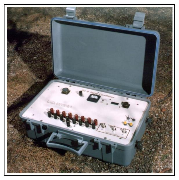
The SC-8 Signal Conditioning Box is used to amplify and filter electric and magnetic telluric signals prior to entering the GDP receiver system. Use of this device is recommended to provide low-noise amplification, radio-noise filtering, and limiting of low-frequency tellurics for MT/AMT surveys. The SC-8 can also be used as a radio signal filter for CSAMT and IP surveys.
