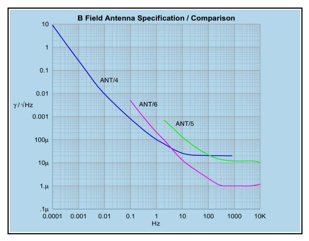
The ANT/4, ANT/5 and ANT/6 magnetic field sensors are extremely low noise instruments. Using feedback amplifier technology and including carefully designed mu-metal cores, these antennas are each designed with specific purposes in mind. Each antenna is designed to be a highly flexible instrument, built to withstand the difficult conditions encountered in the field environment.
