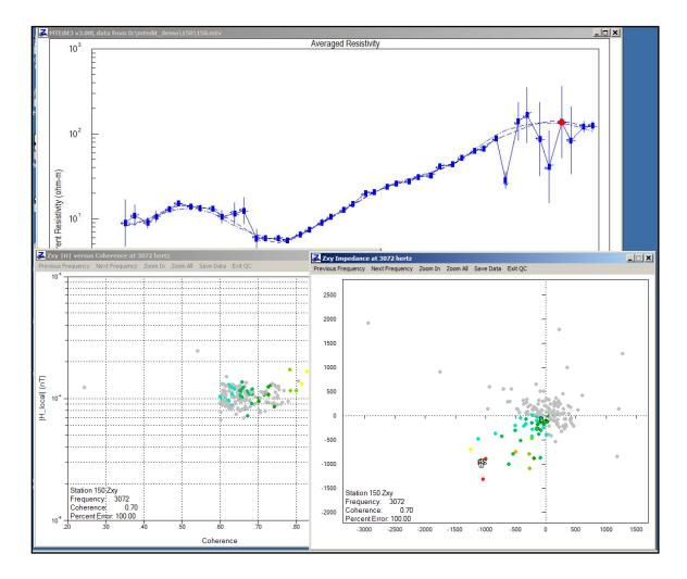
QC editing is most commonly done using the Real(Z) versus Imag(Z) plot. Impedance points are color coded by coherence, ranging from cyan for low to red for high coherence. A  $\oplus$  symbol indicates the robust average impedance value, while PS indicates |Z| from Phase Slope and DP shows the D+ value.
