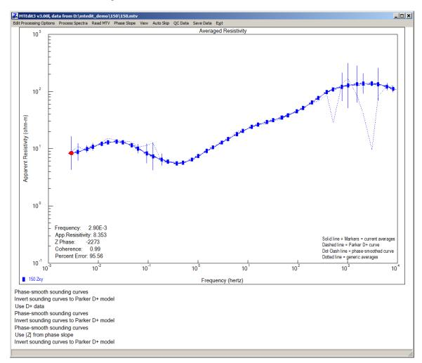
In the example above, the Zxy apparent resistivity for station 150 is loaded from 150.mtv and **Phase** Slope submenu option |Z| from Phase Slope has been selected. The solid blue "active apparent resistivity" curve traces out the |Z| from Phase Slope curve, while the dotted line indicates the more ragged trace of generic robust averaged data.
