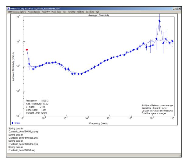
The solid blue line shows the trace of the currently selected apparent resistivity type (generic robust averages, |Z| from Phase Slope or Parker D+). A dotted line indicates generic robust average data, but in the example above generic averaged data are selected, so the solid line overwrites the dotted line. A dot-dash line indicates the **|Z|** from Phase Slope curve and a dashed line indicates the **D+ curve**.
