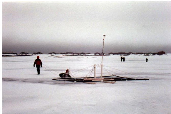
Figure 2: A sled mounted NanoTEM system configured with a 4.6 by 4.6 m transmitter loop and a single 1.5 by 1.5 m horizontal receiver loop for locating UXO on the bottom of a frozen lake. Larger loops were used to improve the response from conductive objects on the bottom of the 6 m deep lake.
