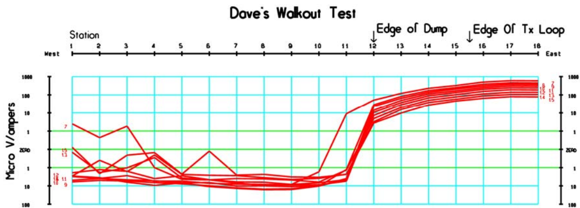
Figure 6: Results from Dave's Walkout Test, windows 7-12, extending from within the dump to several meters away from the edge.
